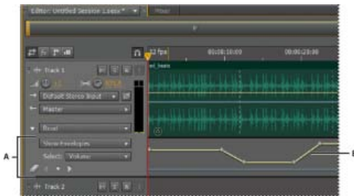
Automating track settings in the Editor panel A. Automation lane B. Envelope for parameter
