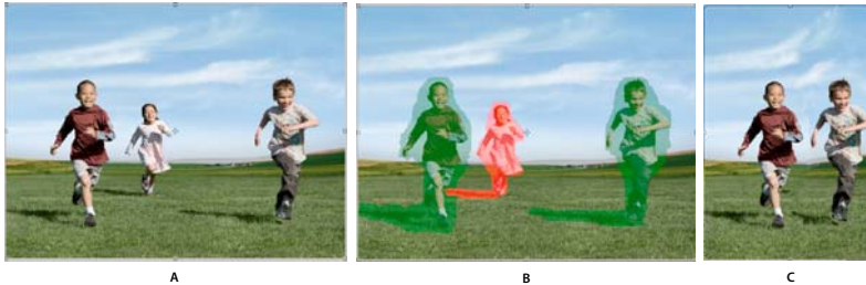
A. Photo selected for Recompose B. Areas marked for protection (green) and for removal (red) C. Photo after Recompose
