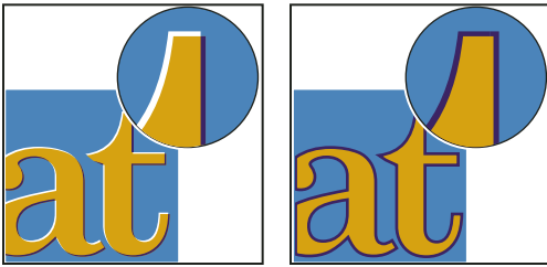
Misregistration with no trap (left) and with trap (right)
