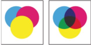
Three overlapping circles without overprinting (left) compared to three overlapping circles with overprinting (right).
