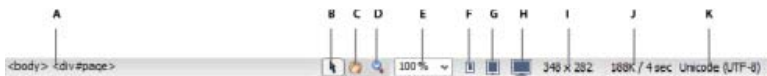
A. Tag selector B. Select tool C. Hand tool D. Zoom tool E. Set magnification F. Mobile size G. Tablet size H. Desktop size I. Window size J. Download size / Download time K. Encoding format
