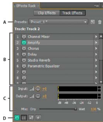
A Rack Preset controls B Effect slots C Level controls D Main Power button
