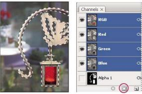
Selection saved as an alpha channel in Channels panel
