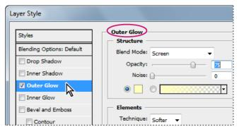
Layer Style dialog box. Click a check box to apply the current settings without displaying the effect's options. Click an effect name to display its options.
