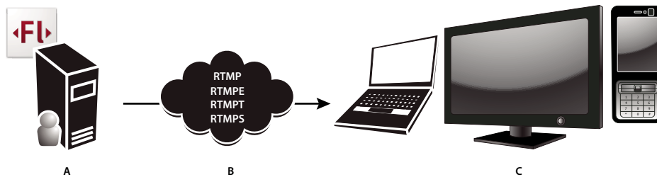
A. Flash Media Server streams recorded media to clients. B. Internet (RTMP, HTTP) C. Flash Player, AIR, iOS devices, and Mac OS stream the video.
