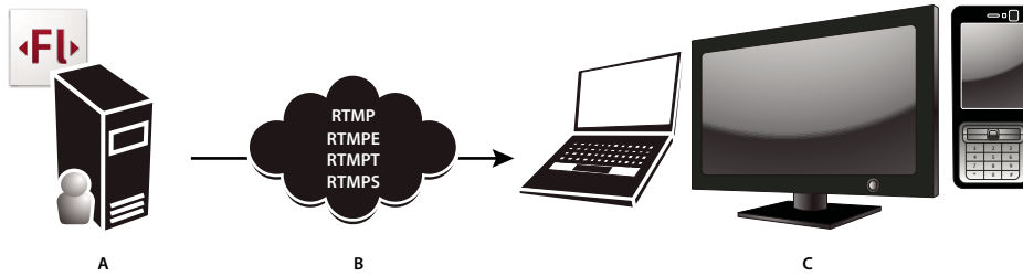
A. Flash Media Server streams recorded media to clients. B. Internet (RTMP) C. Flash Player, AIR, or Flash Lite run the video players
