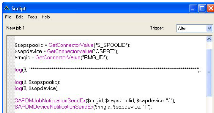
Figure 2 Script storing job and device status, including Output Center status code, in runtime repository.
